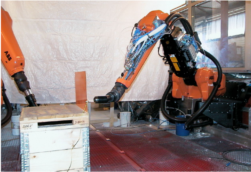
Fig. 4. Setup for experimental testing with paint using ABB robot. Photo courtesy ABB, from [5].
