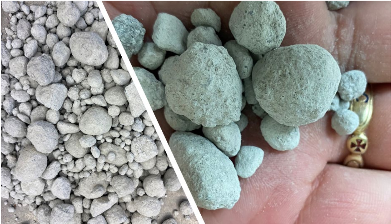
Figure 2 – The RCM-RA in bulk (left) and detail (right), scaled towards a human hand.
