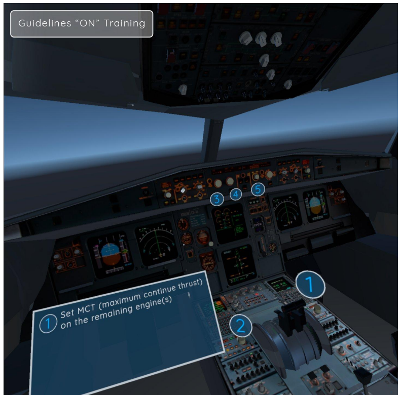
Figure 4.9. Screenshot of the VR procedure trainer of abnormal operations prototype: Guidelines "On"
