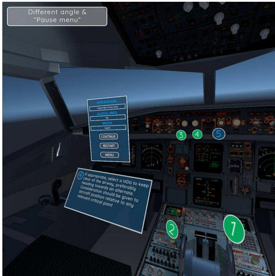
Figure 4.11. Screenshot of the VR procedure trainer of abnormal operations prototype: UI elements
