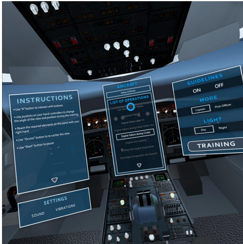
Figure 4.5. Screenshot of the VR procedure trainer of abnormal operations prototype: Main Menu
