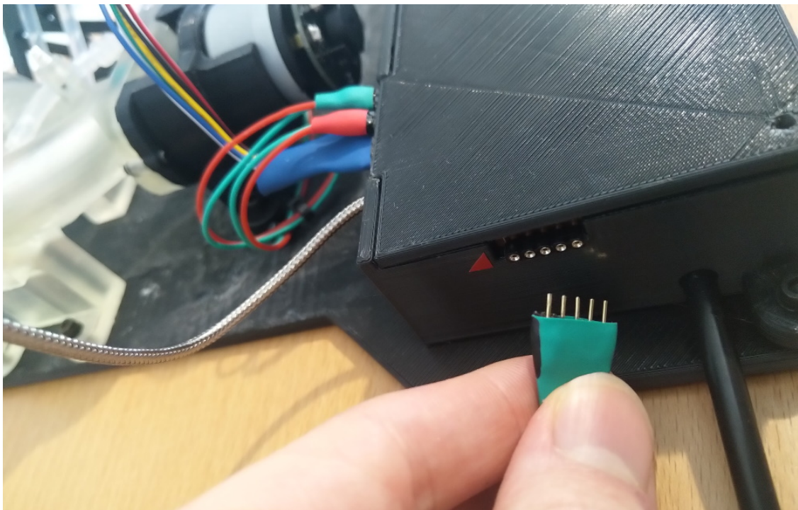
Figure 7.4: Connector style used between external components.
