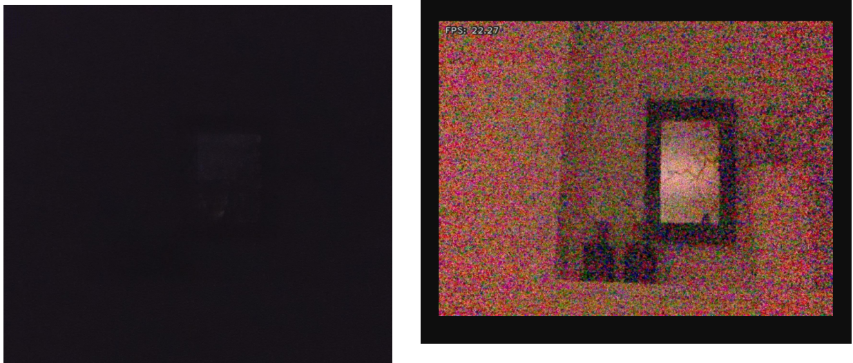
Figure 4.6: The images shows the difference between a regular camera and Raspberry pi NoIR at the same light level. Left: Phone camera, Right: Raspberry Pi NoIR
