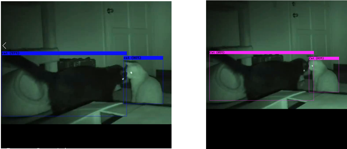
Figure 3.2: YOLOv4 (left) compared with custom training using 2000 images from OID (right)
