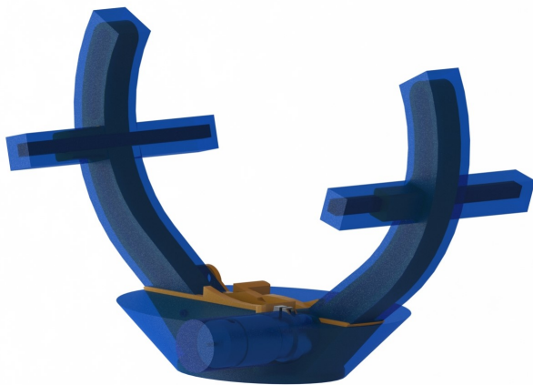
Figure 6.2: Collision geometry of the gripper embracing the more detailed CAD-model
