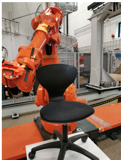
(a) Photo of the robot colliding with the chair
