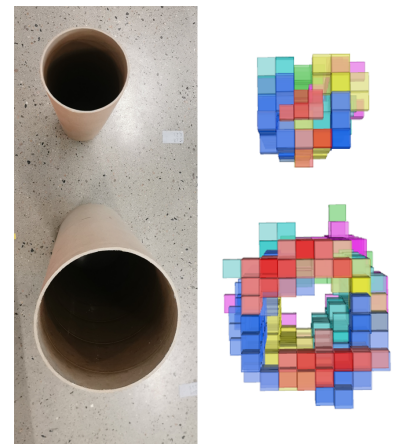
Figure 7.1: The large and the small cylinder shown from above from a photo (left) and a point cloud (right)
