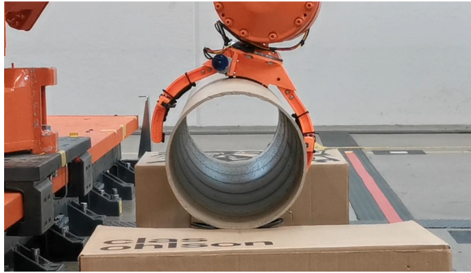
Figure 6.7: Object stand compressed from applied robot force
