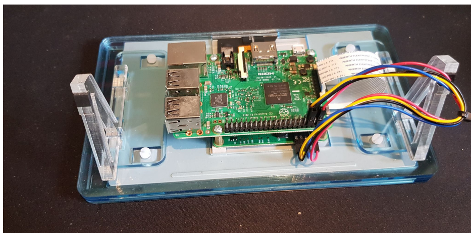
Figure 3.8: Raspberry Pi 3b+ with add-on card and the official raspberry display
