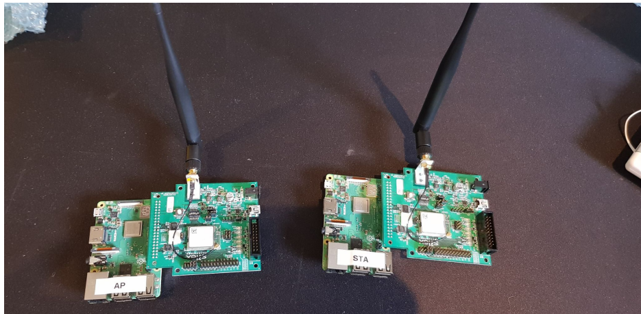
Figure 3.11: Two evaluation kits used to test Wi-Fi HaLow
