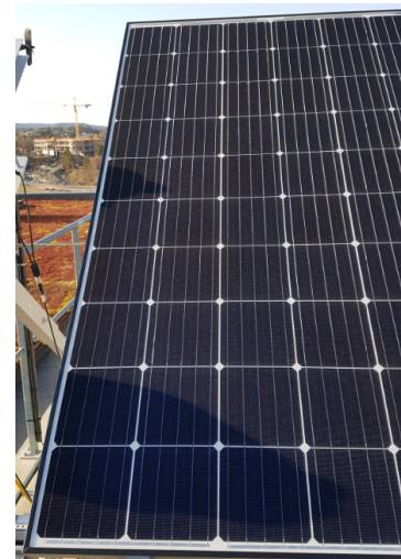
Figure 6.3: Picture of the shadow on the 45^\circ tilt mono c-Si module at 5pm.
