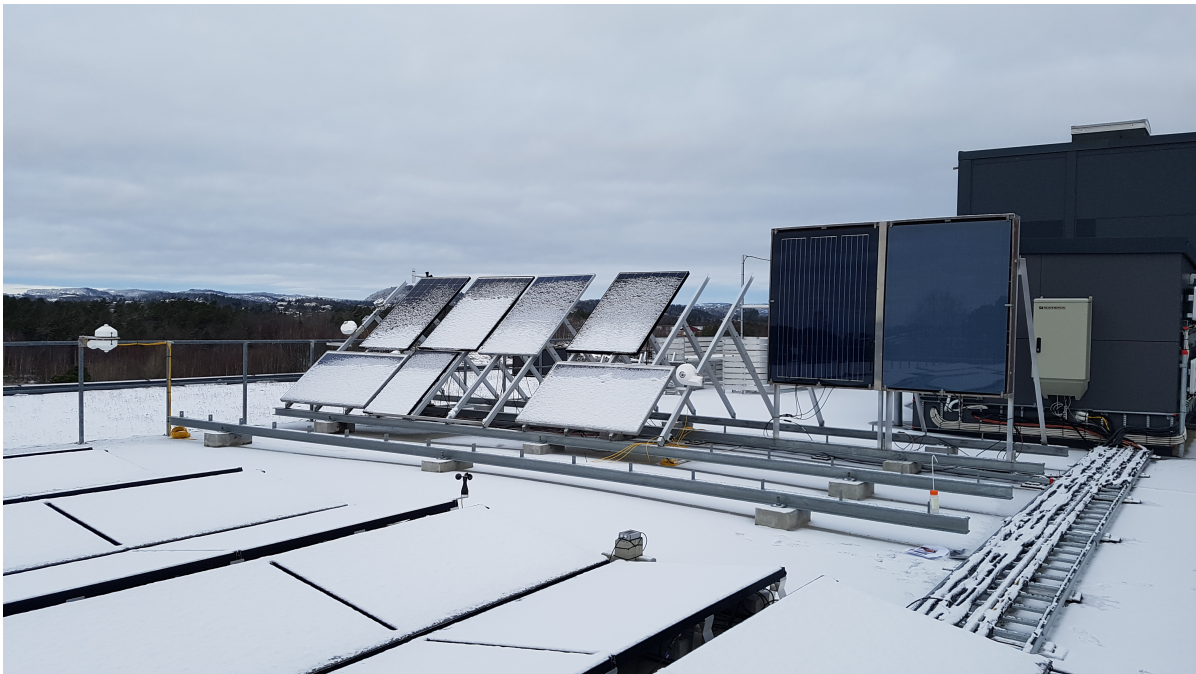
Figure A.2: Picture of the 45° rack covered in snow in January 2021. The BIPV modules are not effected by the snow.
