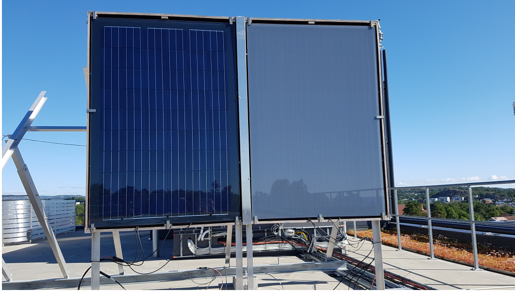
Figure 4.5: Picture of the normal BIPV (left) and the grey BIPV (right) modules mounted at a 90° tilt.
