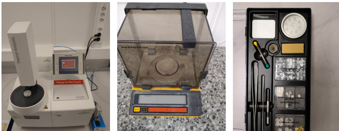
Figure 19 – From left: TGA-1-HW, separate weight used when distributing samples, kit to distribute samples and crucible.
