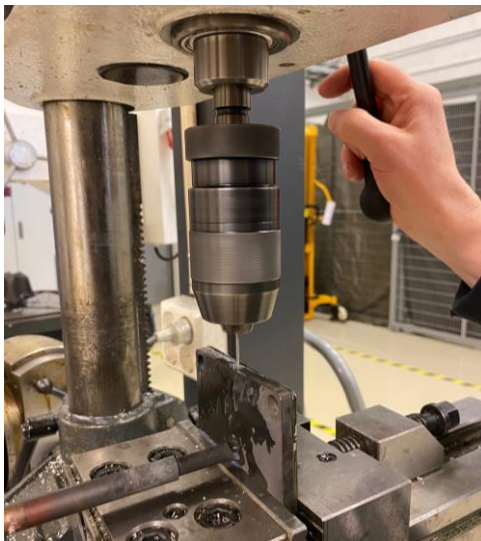
Figure 23 Drilling hole to reconnect the nickel wire
