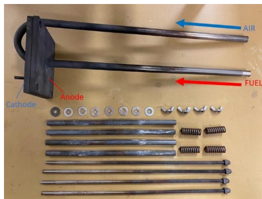
Figure 28 Metal flange housings with rods, springs, nuts and stop washers disassembled
