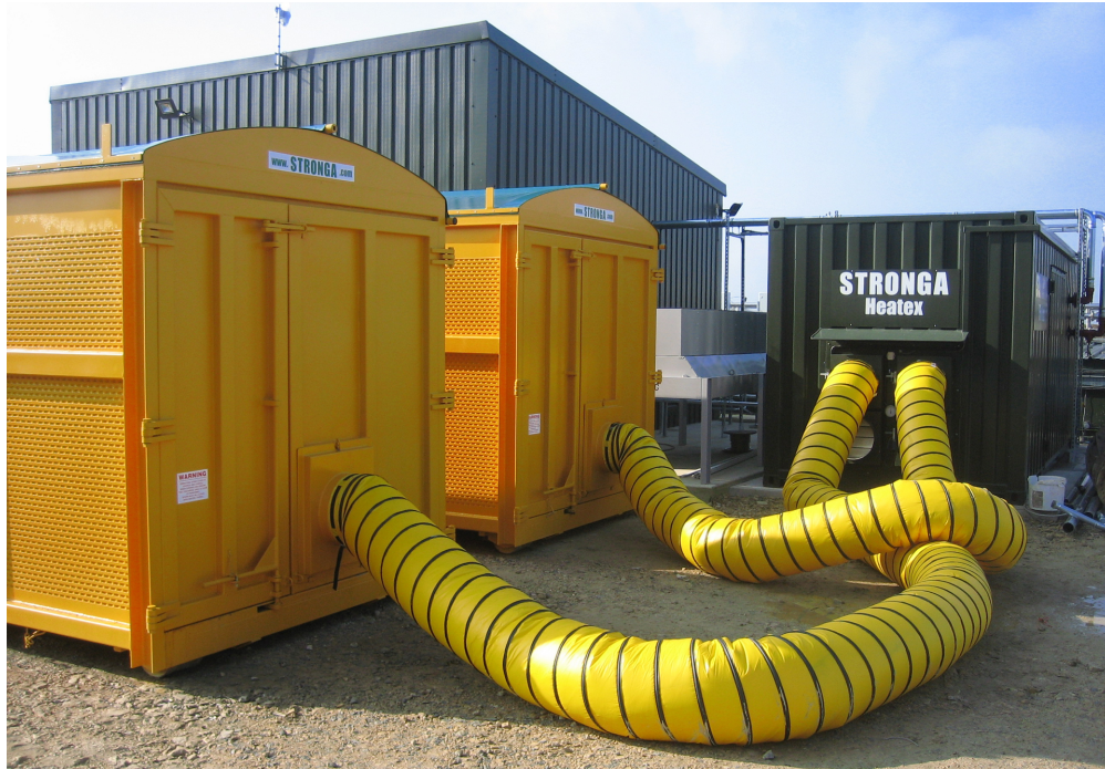
Figure 5.2: Container drying of wood chips [62]
