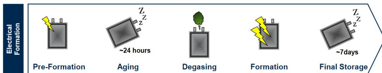
Figure 4.6: Electrical formation stages [43]
