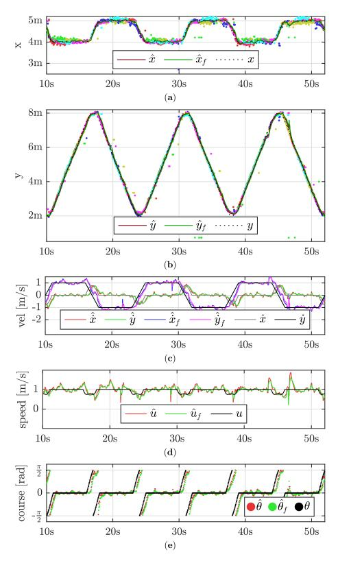
Figure E.3: Timeplots of outputs from the AKF compared to the reference shown in black. Position estimates for x and y are shown in (**a**) and (**b**), respectively. Here, detections are included according to legend in Figure E.2, but not shown in the respective legend. Velocity is shown in (**c**), speed in (**d**) and course in (**e**) where direction is positive clockwise from positive (and negative) y-axis.
