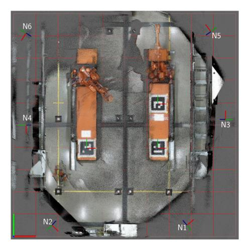
Figure E.1: Orthogonal view of a combined point cloud depicting the Industrial Robotics Lab at the University of Agder. Sensor node poses are annotated N1-N6. The sensors are located 4.3 m above the floor and are angled approx.  $60^{\circ}$  from horizontal. The origin of the world frame is located at the bottom-left, where the red and green lines represent the X and Y-directions, respectively.
