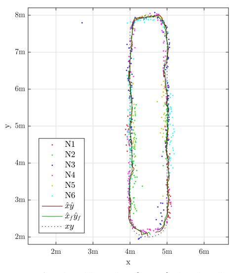
Figure E.2: Positions from the middle round, t = [10 s, 24 s], where the walking pace was 1 m/s in clockwise direction. Detections from sensors N1-N6 are illustrated using dots in separate colors. Red and green line show the estimated position and EWMA-filtered position, respectively. The dotted line is the reference.
