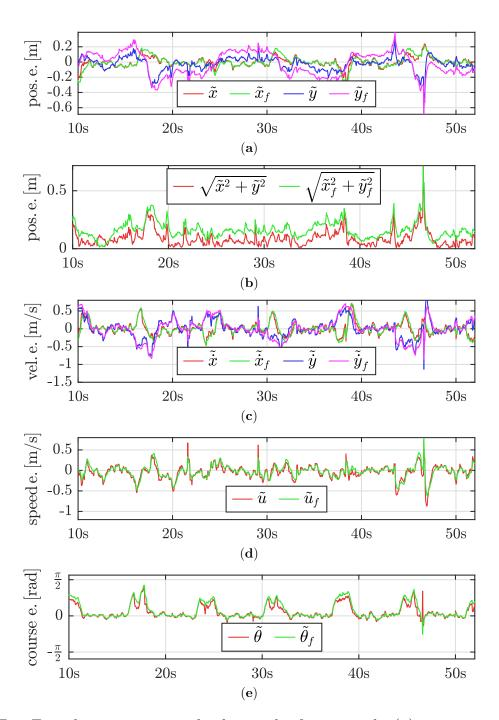
Figure E.5: Error between estimated values and reference path. (a), position error in xand y-direction. (b), Euclidean distance error. (c), velocity error in x- and y-direction. (d), speed error. (e), course error.
