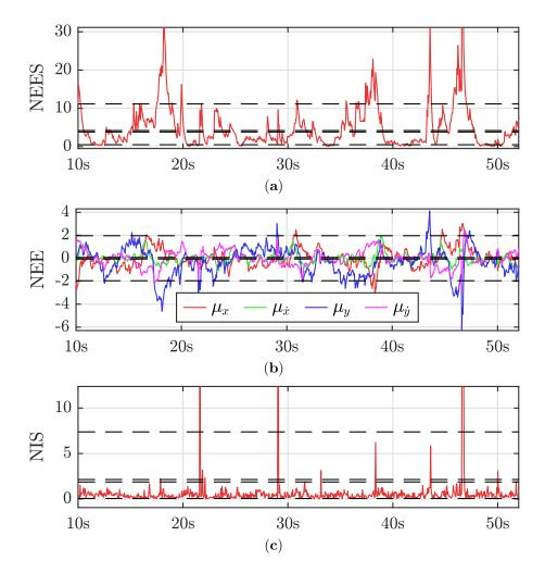
Figure E.4: Statistical tests of the AKF with the two-sided 95% confidence region for a single sample and 840 samples average. (a) show the single run NEES, (b) illustrate the single NEE for the evaluated states and (c) show single run NIS.
