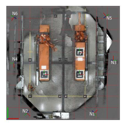
Figure D.2: Overhead view of the combined accumulated RGB point clouds of all six sensors after calibration. Sensor node poses are annotated N1-N6. The sensors are located 4.3 m above the floor and are angled approx.  $60^{\circ}$  from horizontal. The origin of the world frame is located at the bottom-left, where the red and green lines represent the X and Y-directions, respectively.
