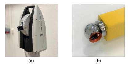
Figure D.3: Leica tracker AT960 (**a**) and Leica SMR Ball Probe (**b**)
