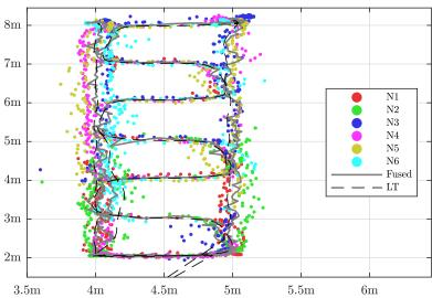
Figure D.11: Walked human path in XY plane at velocity 1.0 m/s using six sensor nodes N1-N6 and depth/YOLO (colored), averaged path (grey) and laser tracker.
