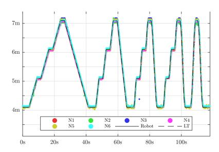
Figure D.4: Robot trajectory in Y-direction measured by the six sensors N1-N6, trajectory via robot and track resolvers and laser tracker.
