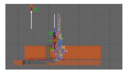
Figure D.7: 6 voxel maps on robot model at velocity  $1.5 \,\mathrm{m/s}$
