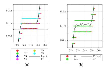
Figure D.5: (a) Selected section of Y-Position measured by 6 sensor nodes, robot position via resolvers and laser tracker. (b) Concatenated N1-N6 (red), the same with latency offset  $\Delta$  (green), concatenated and offset values with moving average filter (grey) and laser tracker (dashed).
