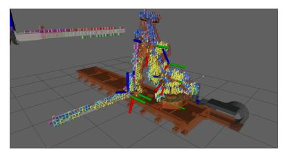
Figure D.6: 6 voxel maps overlaid on robot model at zero velocity.
