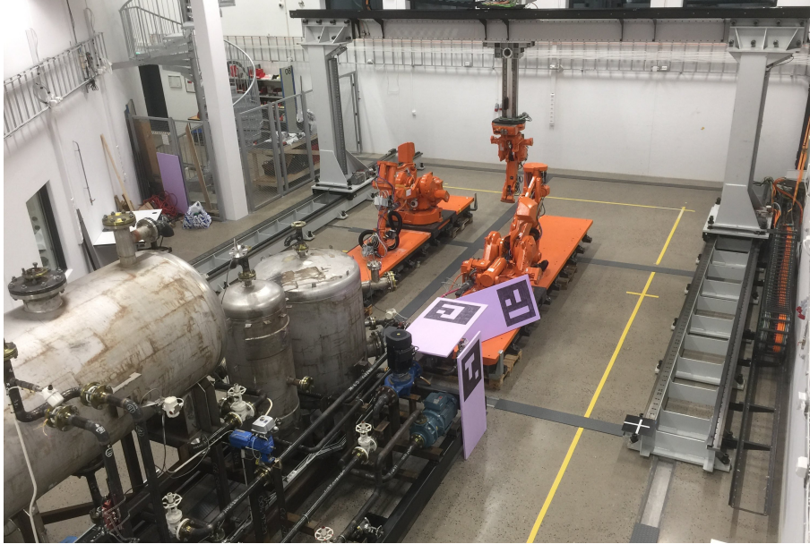
Figure A.1: A Robotics Lab at the University of Agder is used as the example case of an industrial environment. The lab consists of two rail-mounted ABB IRB4400 robots, one ABB IRB2400 robot mounted on a GÜDEL gantry and a processing facility.
