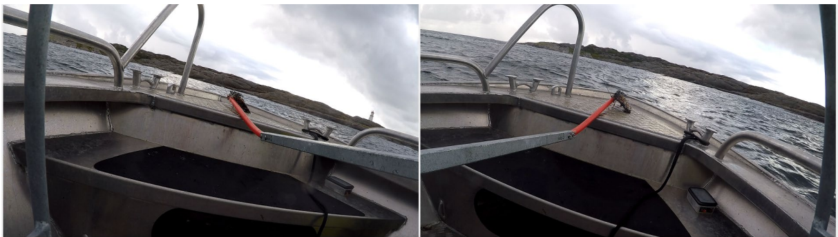
Figure 3.2 Stereo Baited Remote Underwater Video (BRUV) setup: a metal rig with two GoPro cameras with a bait arm in the center
