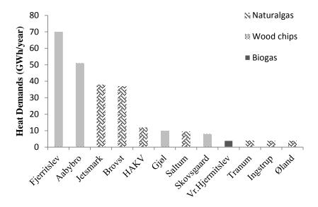
Fig.1: Heat demand and primary fuels for the 12 district heating plants in Jammerbugt municipality.
