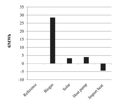
Fig. 8: Variation of heat production price according to different fuel options
