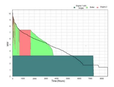
Fig. 7: Duration curve of heat demand and production.
