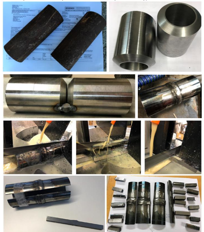
Figure 2. As-received pipe, welding preparation and sample cutting
