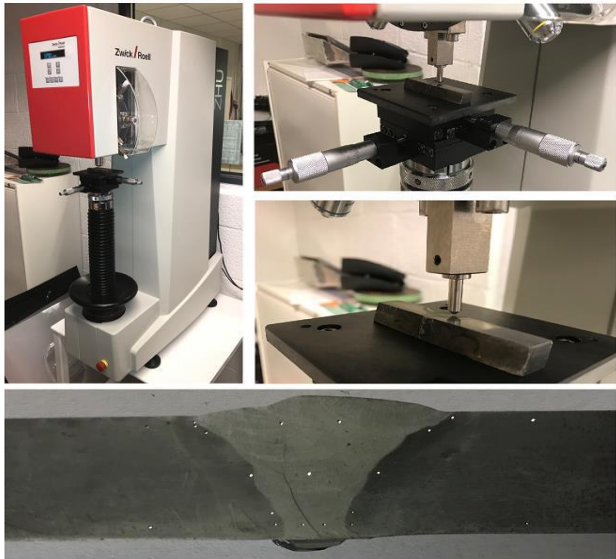
Figure 6. Hardness testing and a sample with indentation marks
