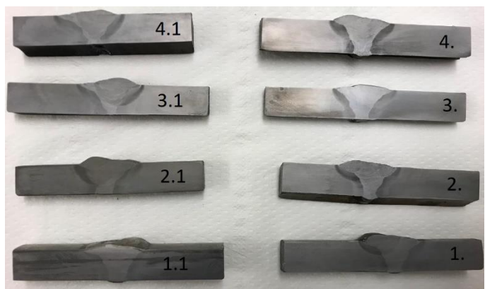
Figure 4. Etched samples for hardening testing
