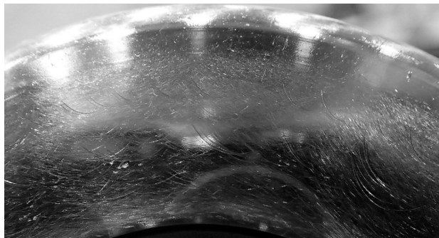
FIGURE 1. Wear on roller end of offshore drilling machine bearing.
