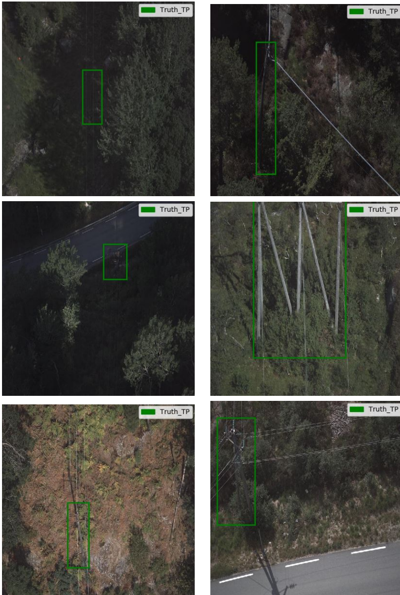
Figure B.1: Pole detection results with no detection of visible poles
