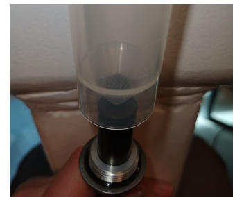
Figure 4.2.: Fine debris calibration with the Gill 4212
