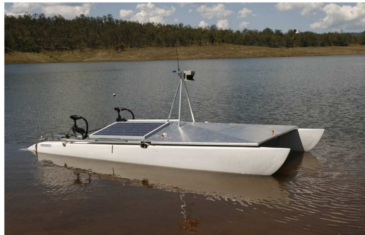
Figure 2.5: Solar powered research USV.
