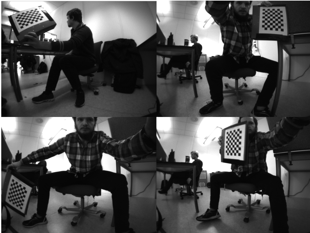
Figure 4.7: Examples of images used in the camera calibration
