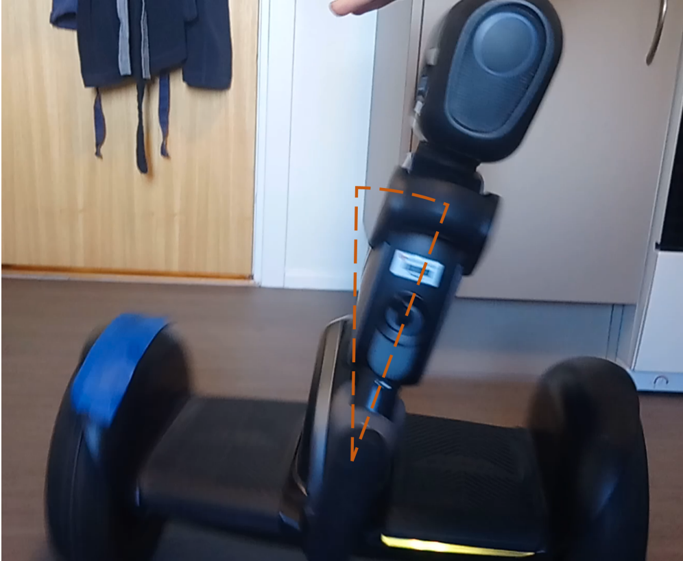
Figure 4.2: When the Loomo is driven manually, turning is done by tilting the upper body of the Loomo
