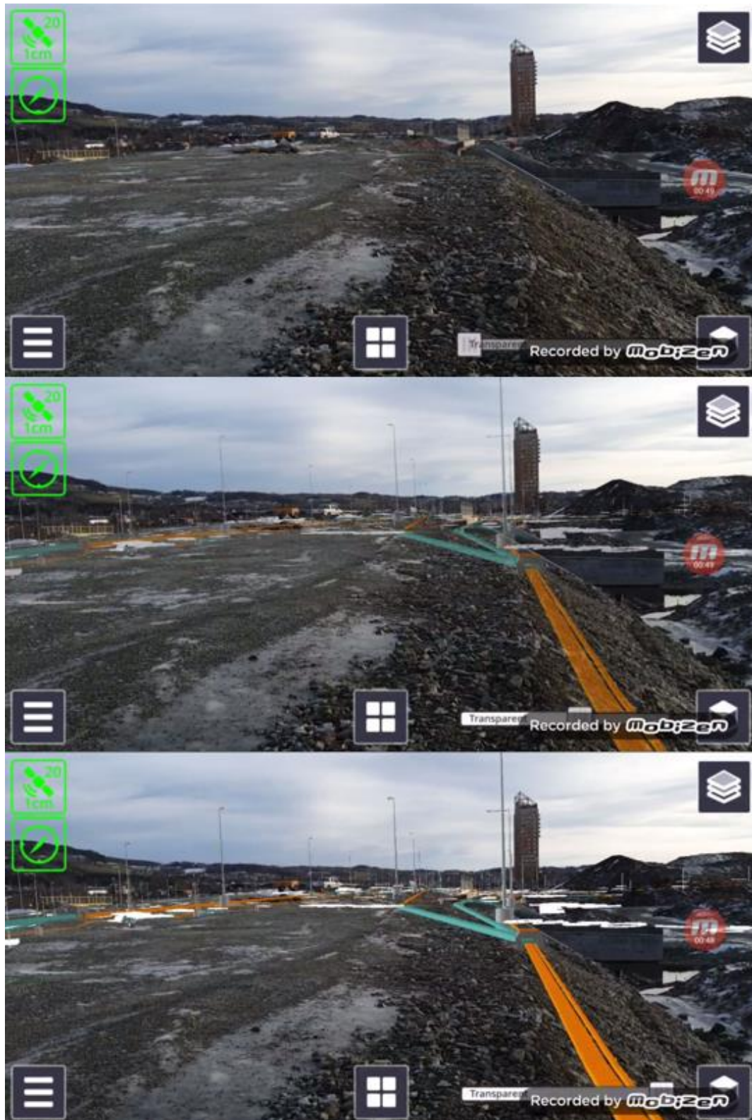
Figure 60 Light posts with foundations and cable trenches visualized over the construction site. The authors have attempted to also show the transparency function of TSV ( Appendix – D.2).
