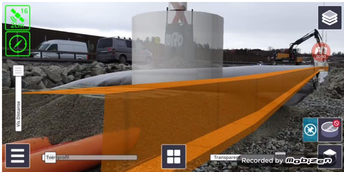
Figure 62 Light post foundation and cables visualized over the real world. Notice how one quite quickly understands that the constructed elements are in accordance with the model ( Appendix – D.2).
