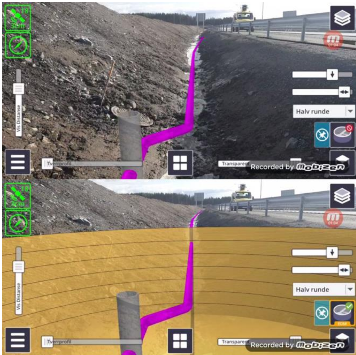
Figure 55 Water installations visualized over the real world. One quite quickly understands that the constructed elements are in accordance with the model. Notice the lines in the “pit” quickly telling the viewer that the pipes are approximately 120cm below ground ( Appendix – D.2).
