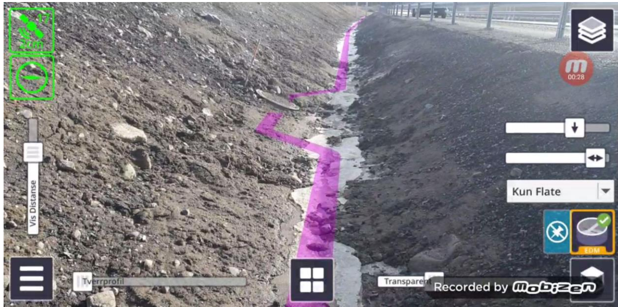
Figure 63 Pit View only surface is used to drape the underground utilities on the surface. One can see how the pipes are centered in the trench and that the manhole is about right ( Appendix – D.2).
