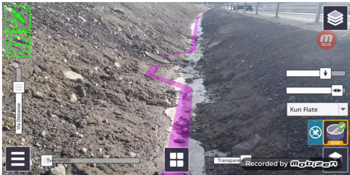
Figure 68 Underground water utilities visualized using the Pit View only surface function in TSV ( Appendix – D.2).
