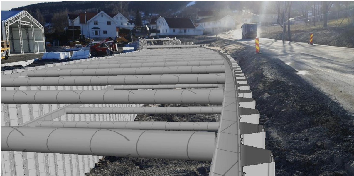
Figure 52 Virtual Sheet pile in gray placed at the construction site ( Appendix – D.2).
