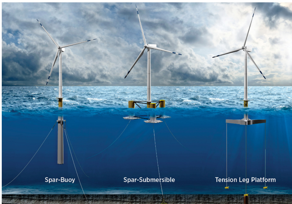
Figure 1.1: Illustration of offshore wind floating foundation concepts [1].
