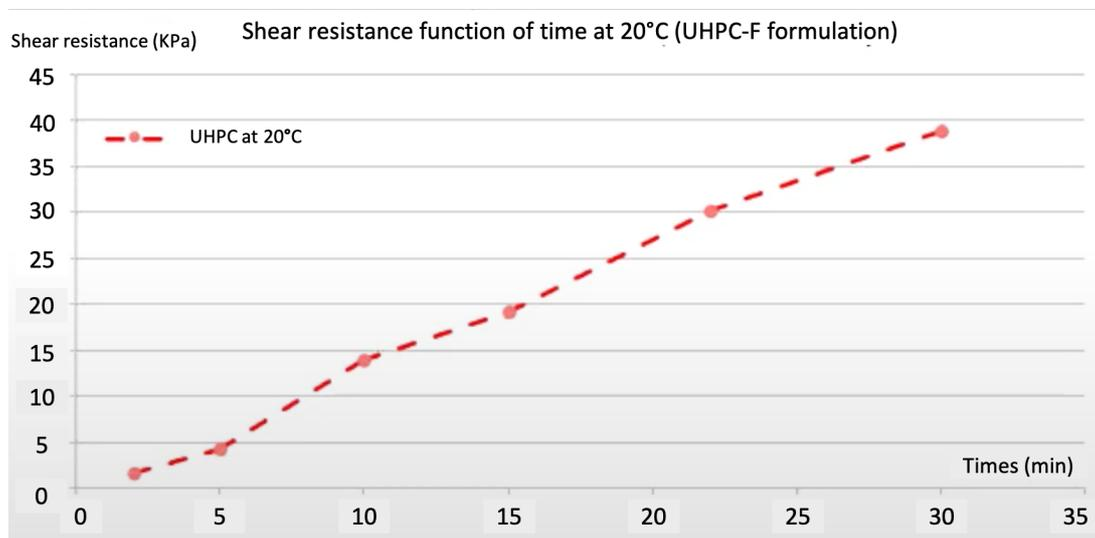
Figure 7.29 Shear resistance, UHPC [94].
