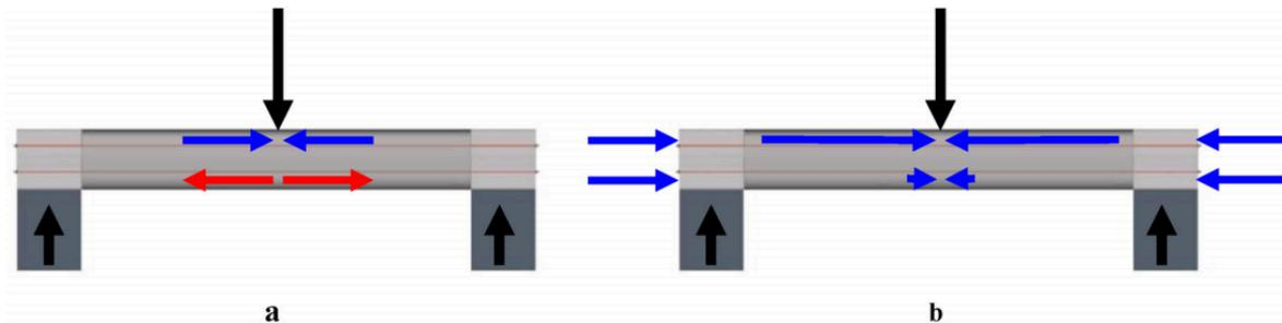
Figure 7.32 Principle of pre-stress applied to a structure loaded in bending. (a): no pre-stress, only bending, (b): pre-stress and bending: the tensile stress in the bottom of the structure is eliminated [49, p. 224].
