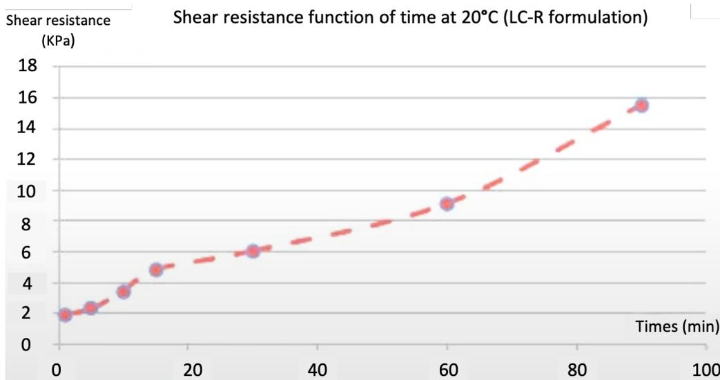
Figure 7.31 Shear resistance, Low-Cost Formulation [94].
