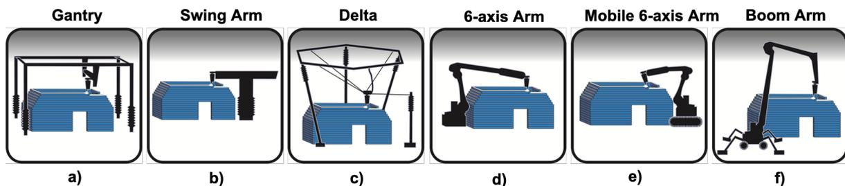
Figure 7.19 3D Printing Technologies Related to Material Extrusion [27].
