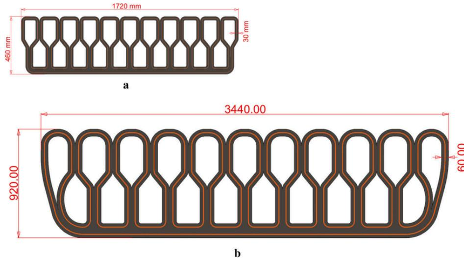
Figure 7.33 Print paths of the 1:2 scale model for testing (a) and the actual bridge section (b). The optimised pattern of the latter with regard to the former saves 4 percent of print path length [49, p. 226].
