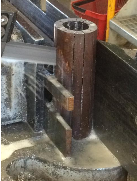
Figure 34: Cutting of the raw steel pipe sample.
