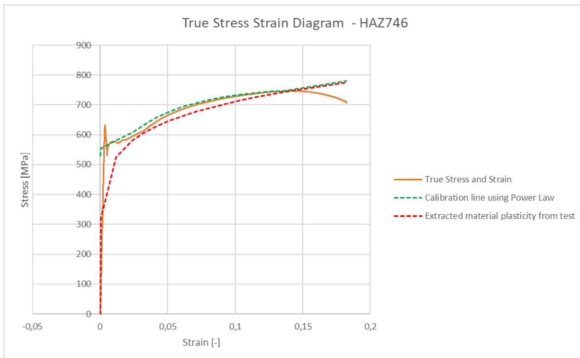
Figure 156: Visualization of calibration of strength coefficient K for the tensile tested HAZ 746.
