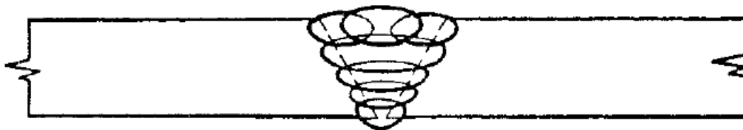
Figure 15: Schematic sketch of multipass welding. Note that the root pass has the highest dilution ratio [13].
