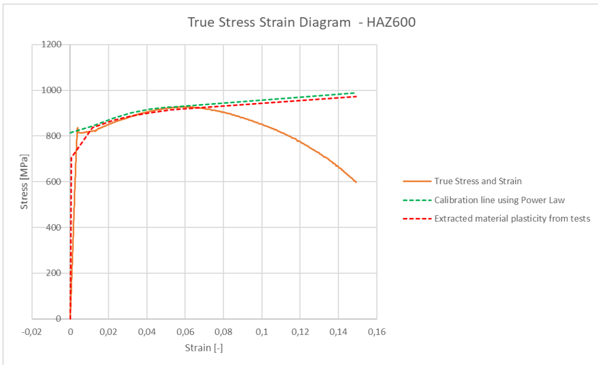
Figure 150: Visualization of calibration of strength coefficient K for the tensile tested HAZ 600.
