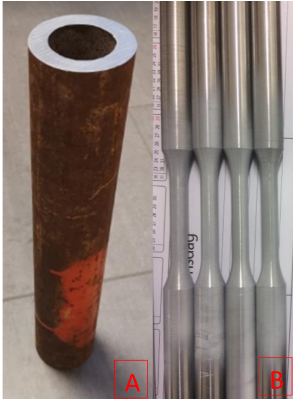
Figure 29: (A) Raw steel pipe sample and (B) Uniform test specimens that were tested in this study.
