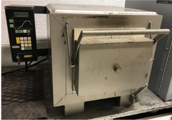
Figure 32: Furnace used for heat treatment of the steel samples.
