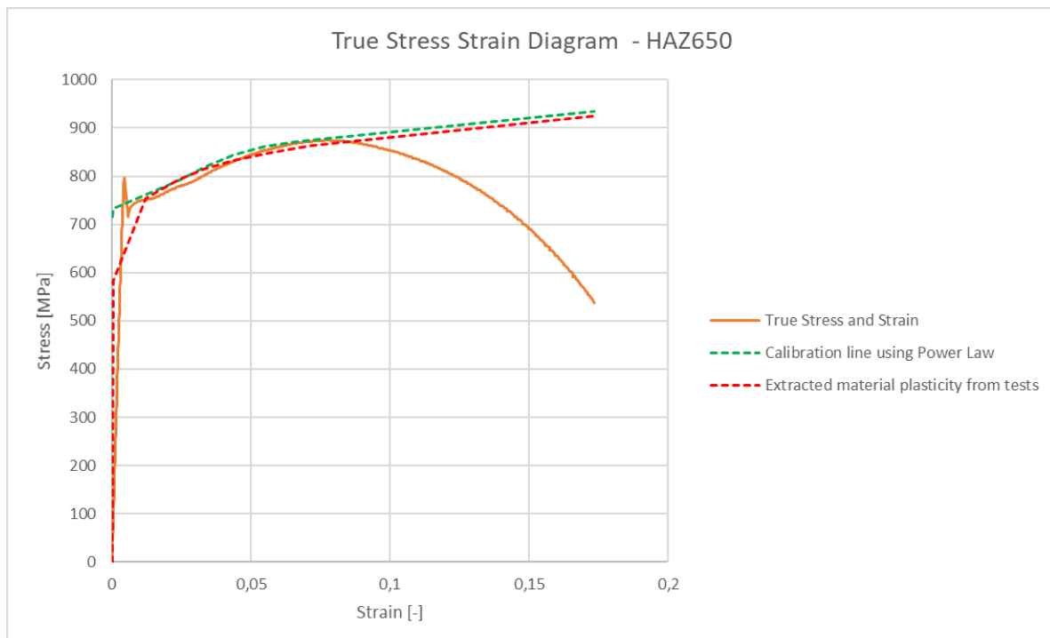
Figure 152: Visualization of calibration of strength coefficient K for the tensile tested HAZ 650.
