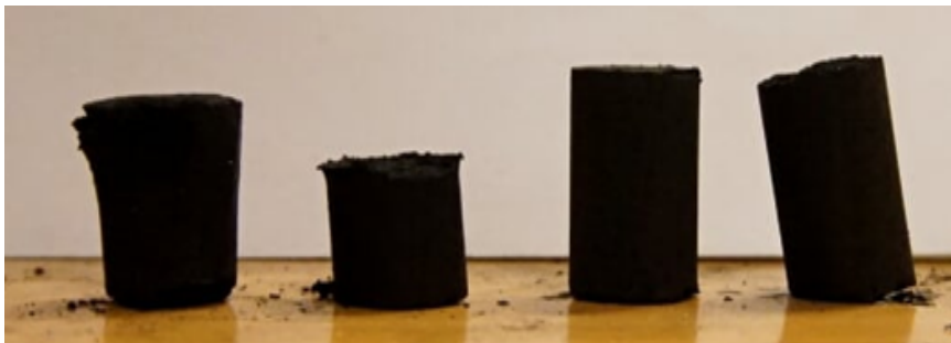
Figure 2.4: Biochar pellets made with a water content of, from left to right, 10, 20, 30 and 40% (total feedstock weight).
