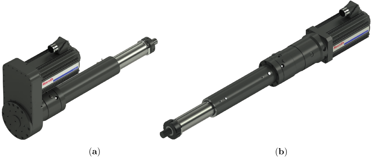
Figure 2.4: Different motor mounting configurations [25]: (a) via timing (gear) belt side drive; (b) directly via coupling.
