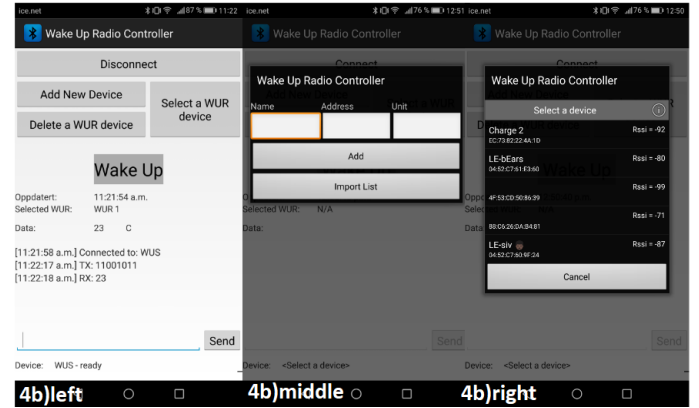
(b) Illustration of data collection in W2B-IoT via an Android APP. 4b)left: User interface and a test result; 4b)middle: Add a new device; and 4b)right: A list of active BLE devices in the vicinity of the WuTx.
