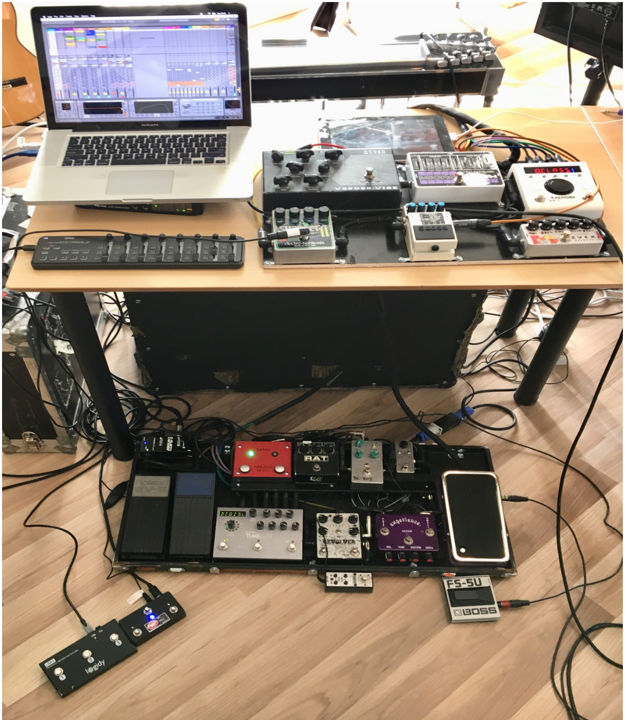
Figure 3: The pedalboards, the computer and the USB controllers. The iPad is the controller for the Eventide H9 connected via Bluetooth. The audio interface, MOTU 4-pre is lying underneath the computer.
