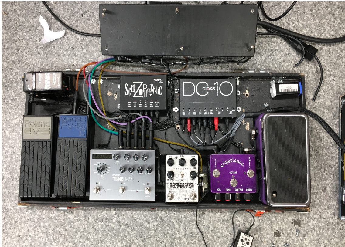
Figure 12: The floor board displaying the two Cioks power supplies. The power supplies are usually hidden.
