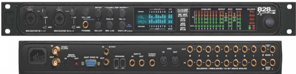
Figure 69: The main audio interface used in my studio
