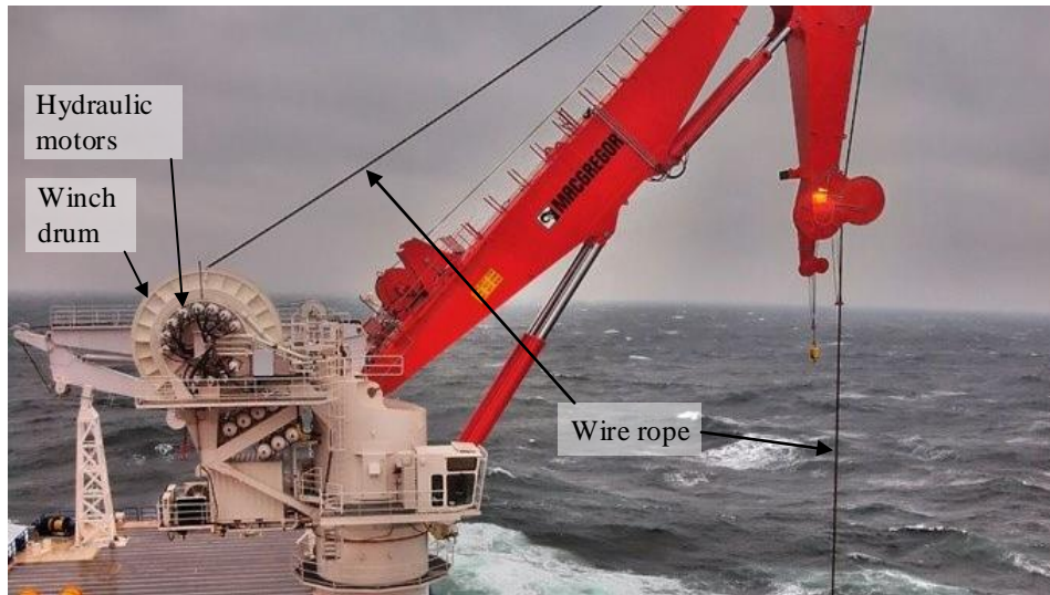
Figure 1.1: Subsea crane equipped with a hydraulic winch system [1].
