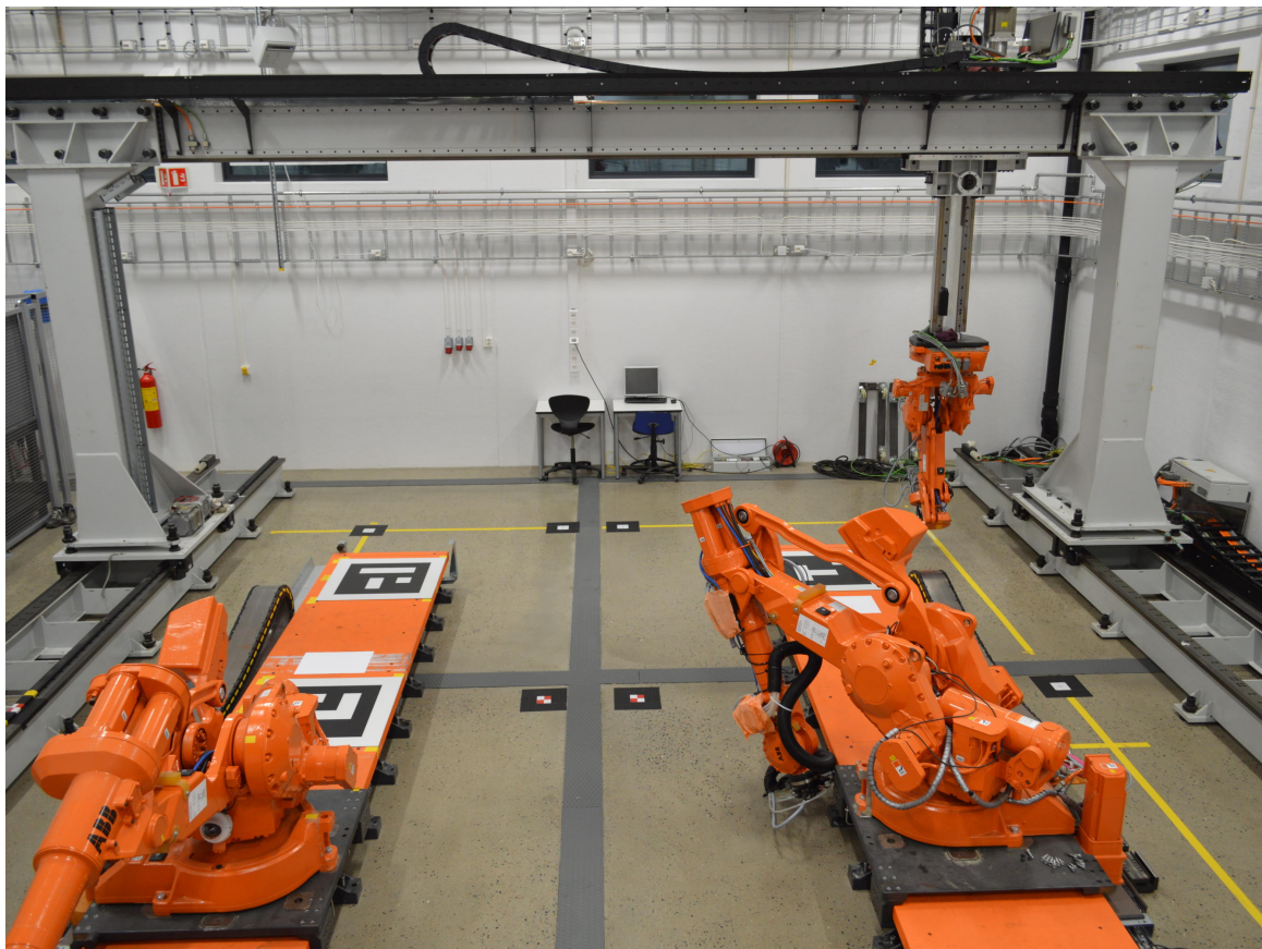
Figure 1. The Industrial Robotics Lab at the University of Agder. This lab consists of two rail-mounted ABB IRB4400 robots, one ABB IRB2400 robot mounted on a GÜDEL gantry and a processing facility.
