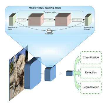
Figure 8: An overview of the MobileNet architecture
