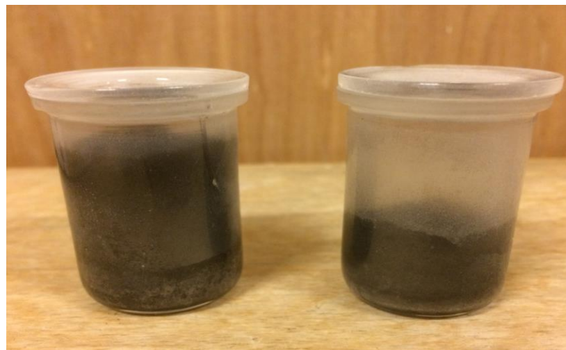
Fig 20: Crucibles with Lid for the VM test for the Alkali lignin and Lignosulfonate
