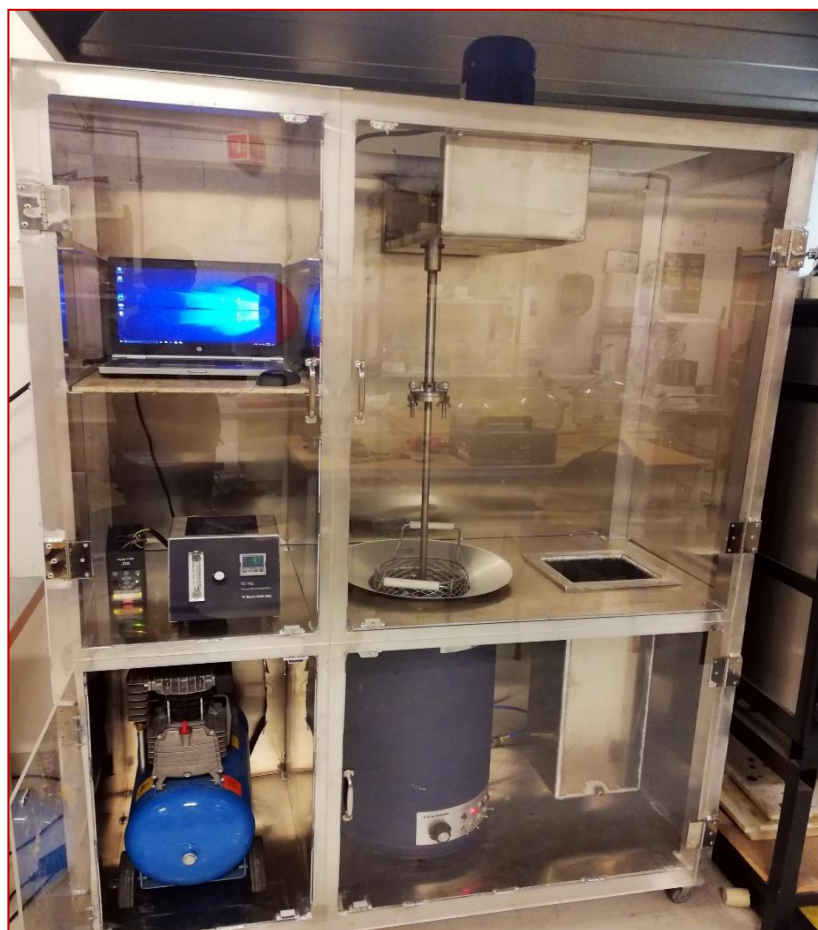
Fig 4: Pilot Hydrothermal Liquefaction Rig Designed and Fabricated by the HTL team
