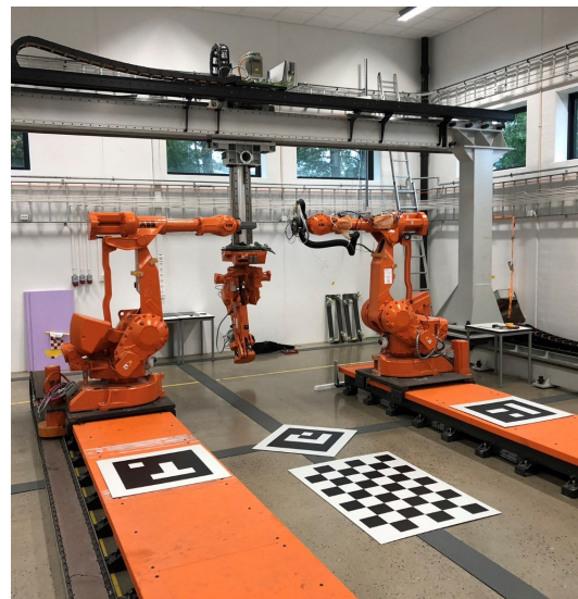
Figure 4. The Industrial Robotics Lab in MIL is used as the example case of an industrial environment. The lab consists of two rail-mounted ABB IRB4400 robots, one ABB IRB2400 robot mounted on a GÜDEL gantry and a processing facility.
