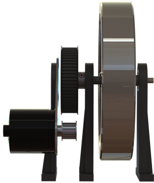
Figure 29: Assembled inertia wheel system
