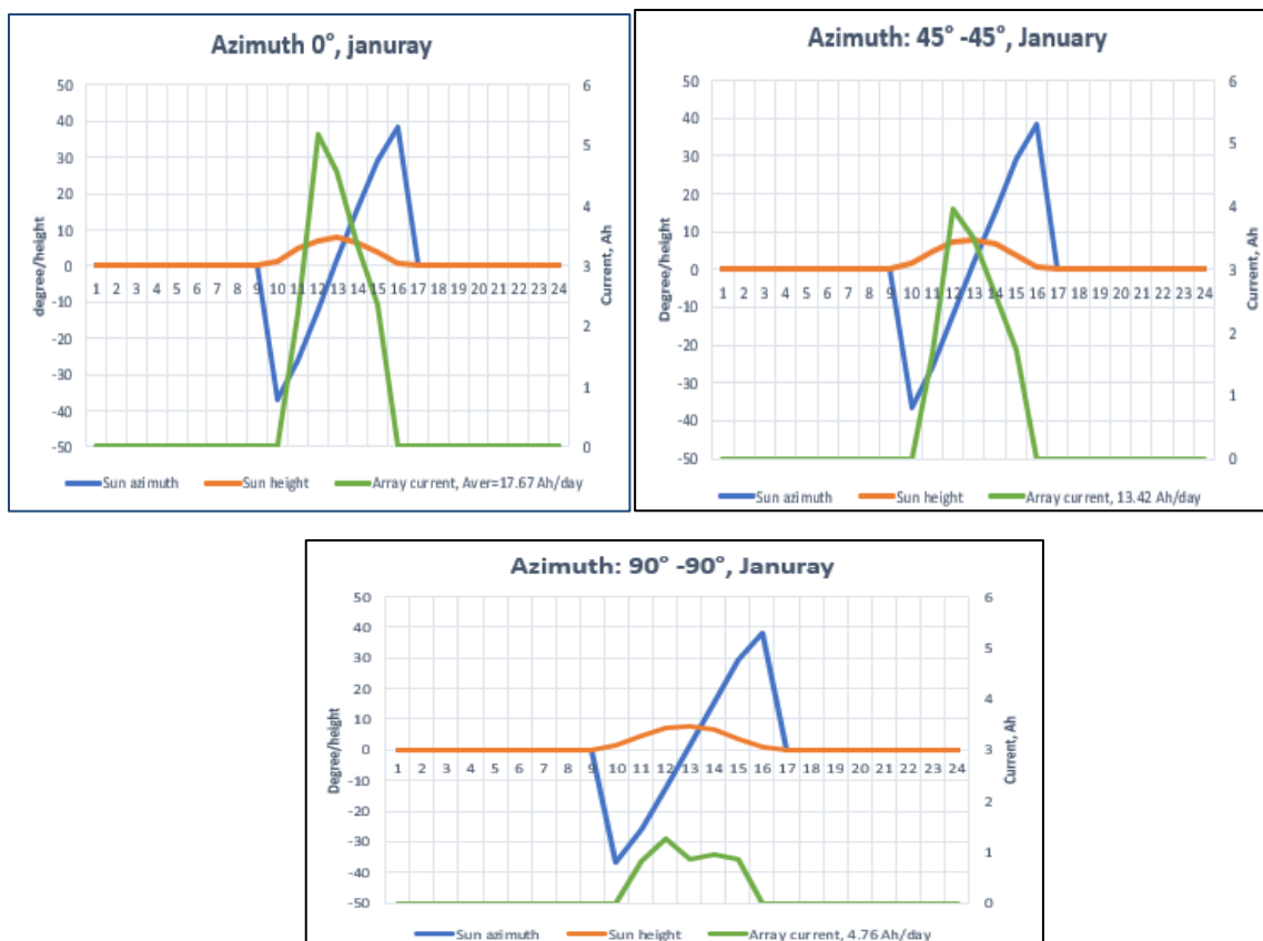
Figure 34 Sun azimuth, sun height and array current for a clear day in January. Three orientations; left graph (south), right graph (southeast and southwest) and bottom graph (east and west). Location: Oslo
