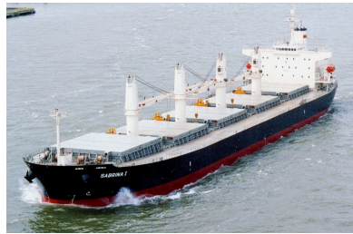
Figure 1.1: Sabrina 1 , a typical, so-called handymax bulk carrier [1].
