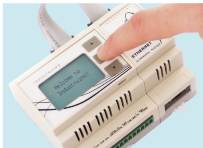
Figure 2.9: Industrino, a fully featured Arduino compatible board [6]
