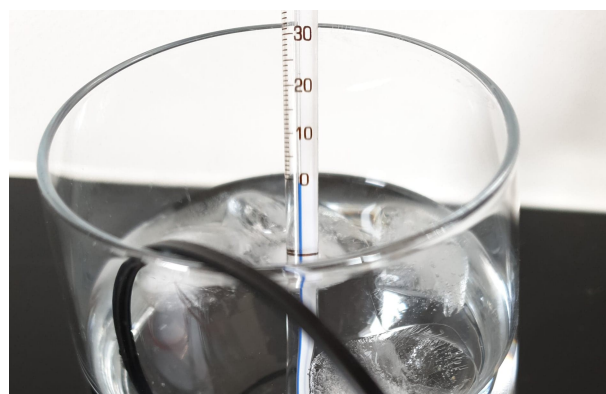
(b) Zoomed in picture of calibration of temperature sensor with 0^\circ\text{C}
