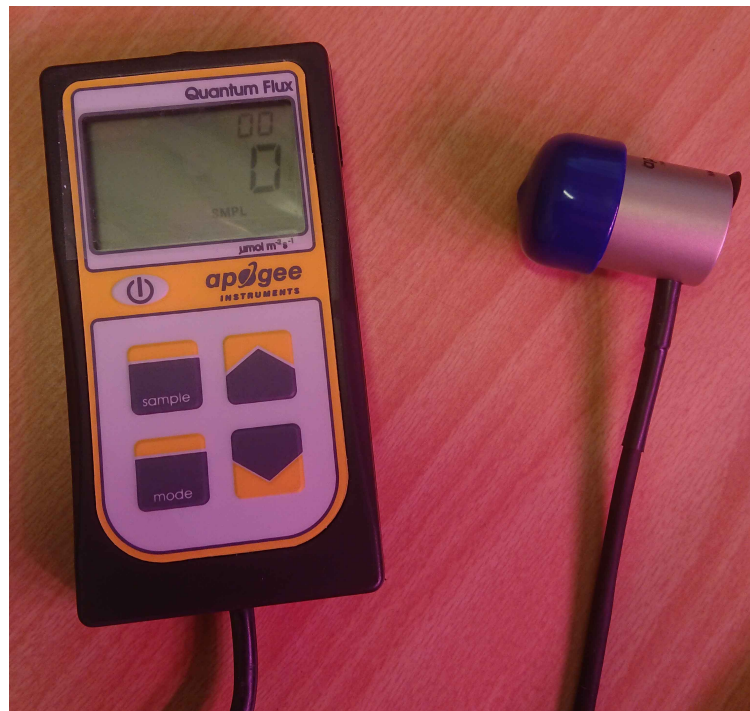
Figure 4.5: Quantum meter with separate sensor from apogee instruments
