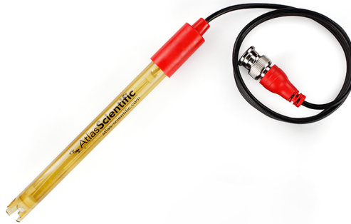
Figure 4.10: pH sensor from Atlas Scientific [9]
