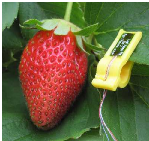
Figure 2.7: Leaf sensor from Agrihouse [4]
