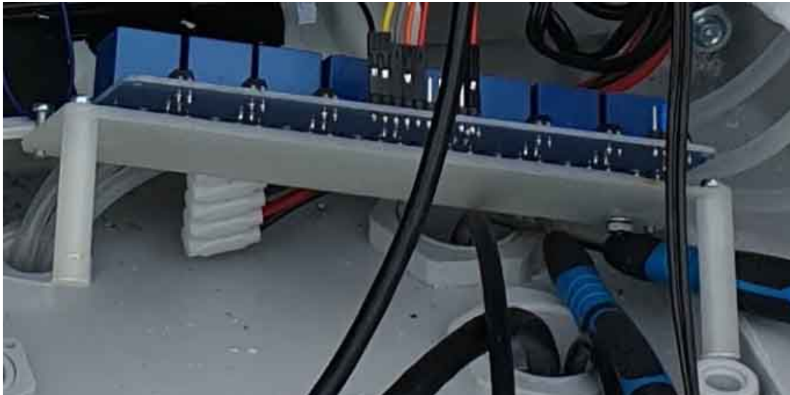
Figure 5.19: Fully assembled bracket with relays
