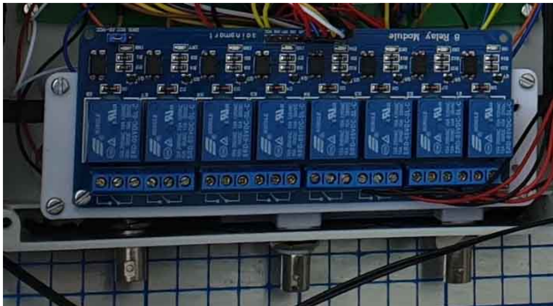
Figure 5.20: Fully assembled bracket with relays attached in the box
