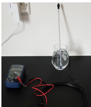
(a) Calibration of temperature sensor with 0^\circ\text{C}
