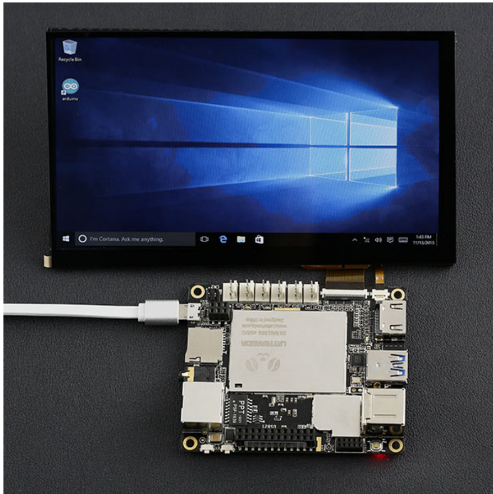
Figure 2.10: LattePanda connected to 7 1024 x 600 IPS display, showing Windows [7]
