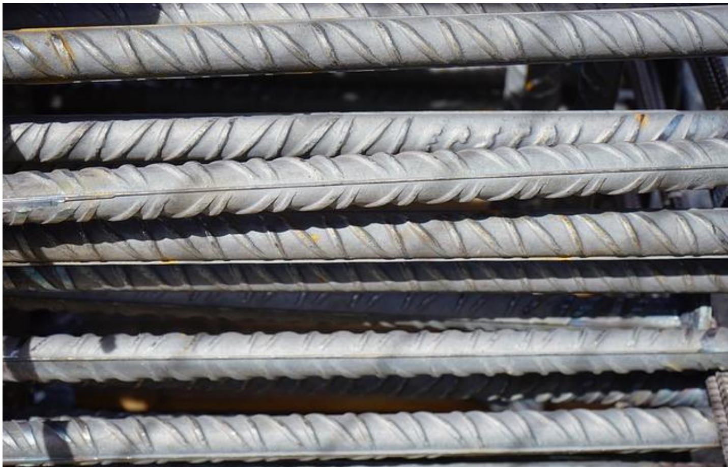
Typical reinforcement bars with ribbed protrusions.
