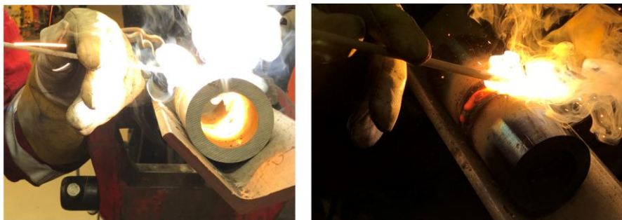
Figure 41, Pictures of welding process. Root and cap welding stages
