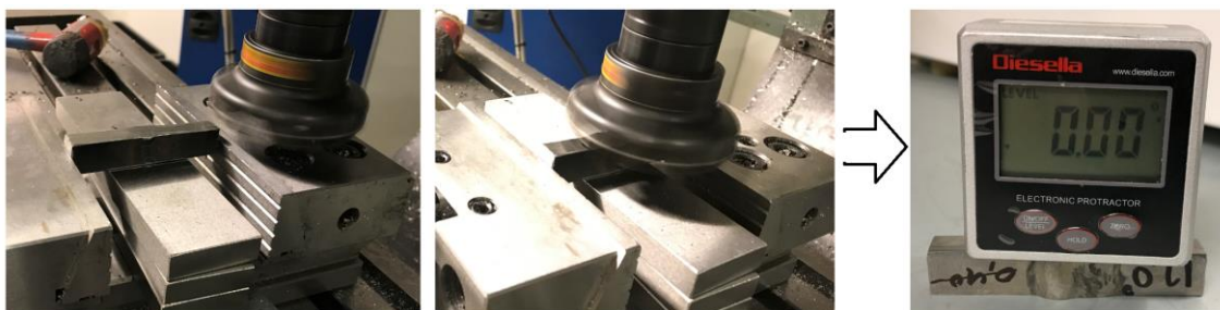
Figure 44, Use of milling machine for surface correction and smoothing
