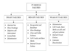
**Figure 2:** Major identified degradation modes of Crystalline PV modules [3]
