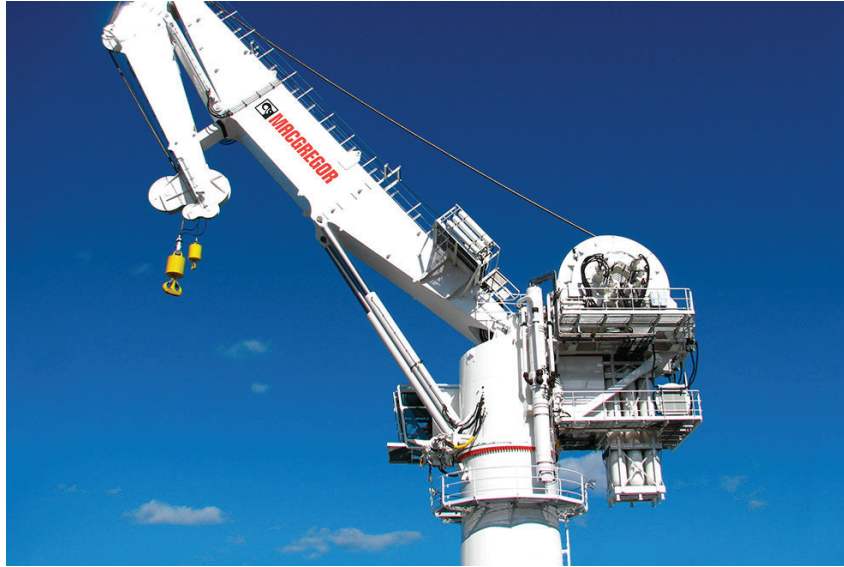
Figure 1.2: An offshore AHC knuckle boom crane manufactured by MacGregor [1].
