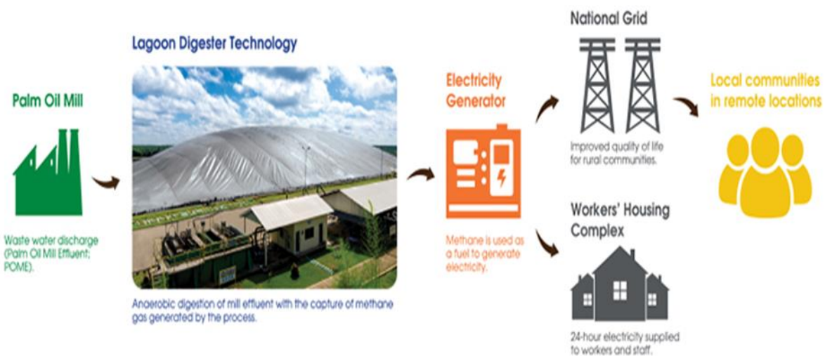
Figure 6: POME to Biogas power generator. (Source: Musim Mas, 2015).
