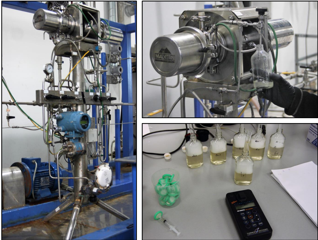
Figure 4.7: Left: Picture of the Insitec installed on a custom-made flow-control assembly. Upper right: Picture of bottle sampling. Lower right: Picture of TD 500D oil-in-water analysis.
