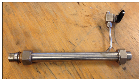
Figure 4.8: Left: Schematics of the isokinetic sampling tubes. Right: Picture of an isokinetic sampling tube.
