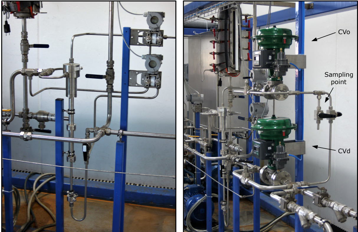
Figure 4.9: Left: Photo of the hydrocyclone mounted in the test rig. Right: Picture of CV_o , CV_d and a sampling point.
