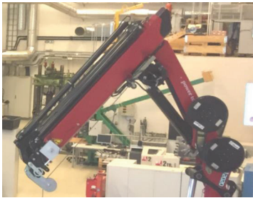
Fig. 4. Experimental setup of the hydraulic loader crane
