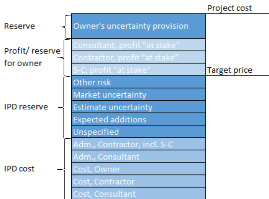
Figure 15 Cost and risk allocation according to IPD model (Tønsbergprosjektet, 2017a, p. 22)
