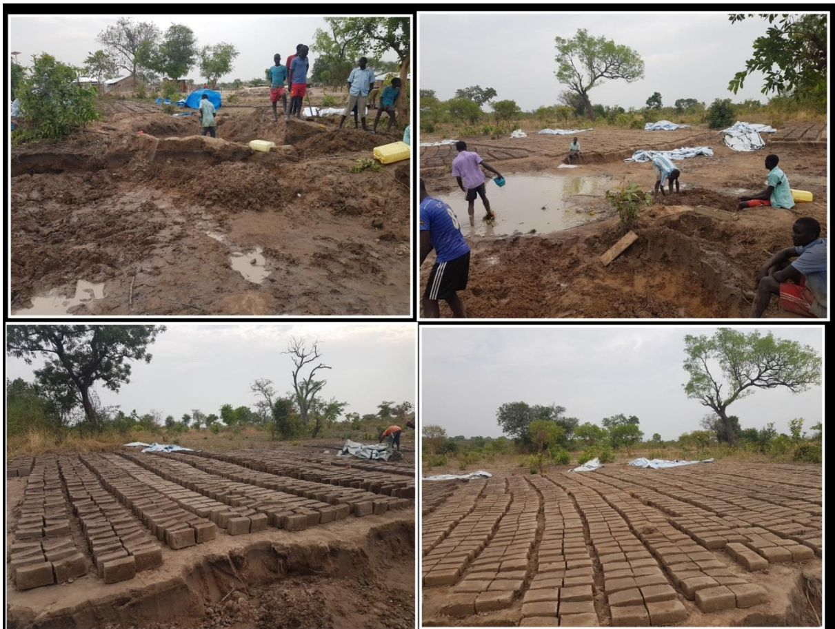
A photo collage showing youths working on brick moulding above and below are photos showing the finished product. Photo: (Tererai Obey Sithole, 2018).
