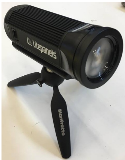
Figure 3.9: One of the three LED lights used to improve camera conditions in this thesis, shown with a tripod mount
