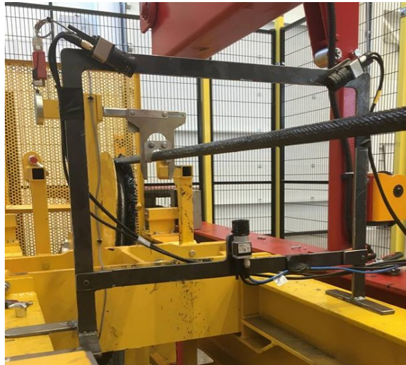
Figure 3.8: The camera system shown mounted to the frame its used with
