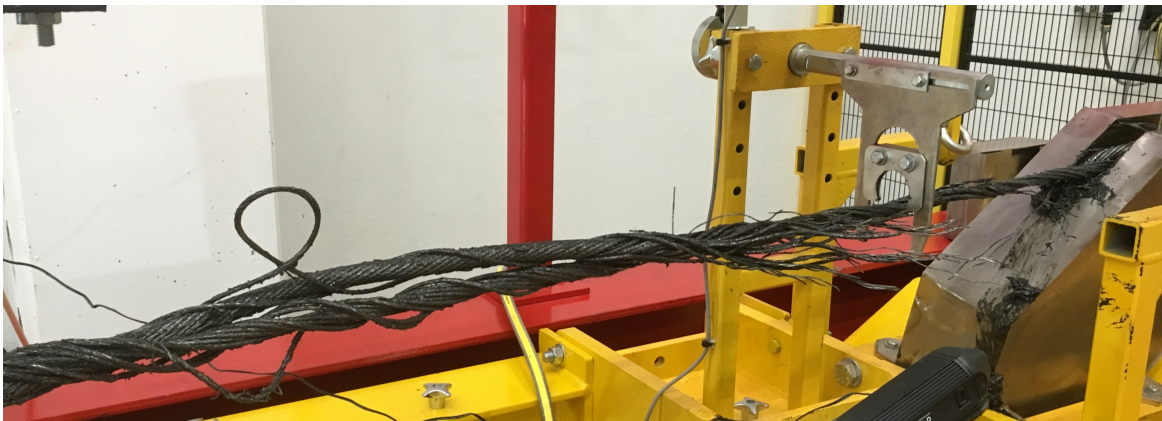
Figure 5.8: A picture of the second rope tested in this thesis subsequent to failure, the rope experienced a rapid and almost total rupture. Prior to this, the measurements of the magnetics tested revealed an exponentially increasing discontinuity, yet the outside of the rope didn't show any obvious signs of such a massive deterioration
