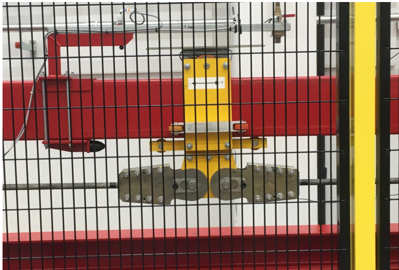
Figure 3.4: The trolley of the CBOS machine shown in its start position with a SWR mounted to it. The machine counts a cycle every time the trolley returns to this position
