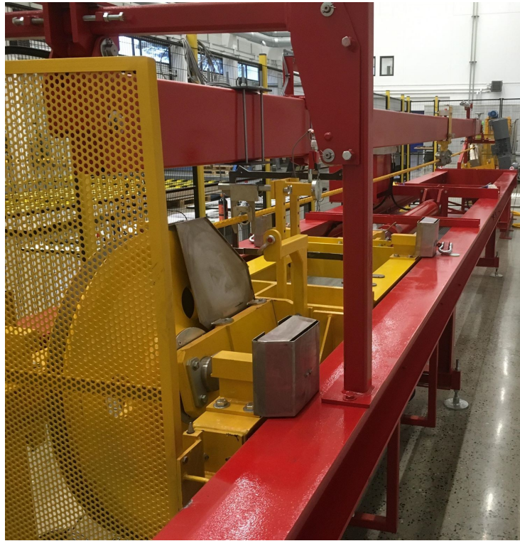
Figure 3.3: The CBOS rope testing machine shown from the backside. The test sheave is visible on the left side. As shown, a yellow fibre rope is mounted at the time this picture was taken
