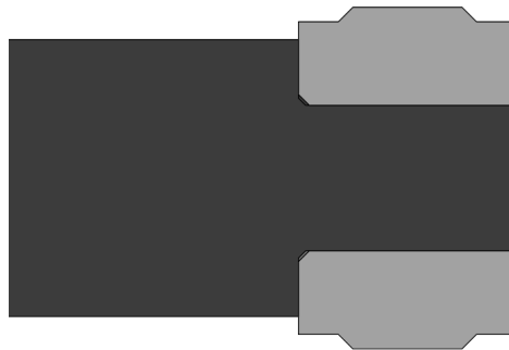
Figure 3.15: Cardan joint link adapter
